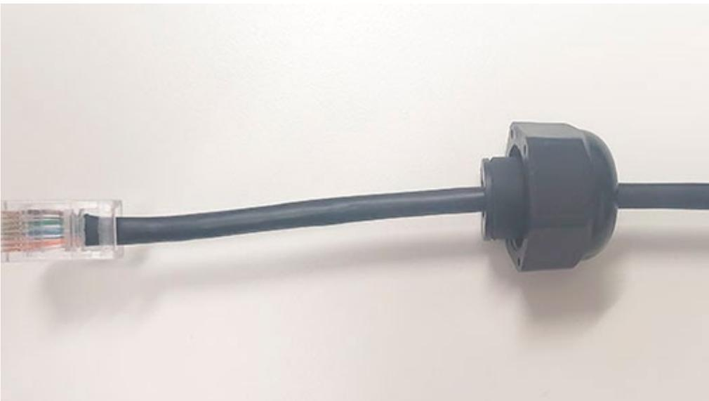
5. Route the Ethernet cable through the small end of the gland base. Align the RJ-45 connector appropriately, then snap the connector into place. Ensure that the connector is fully connected before continuing.
