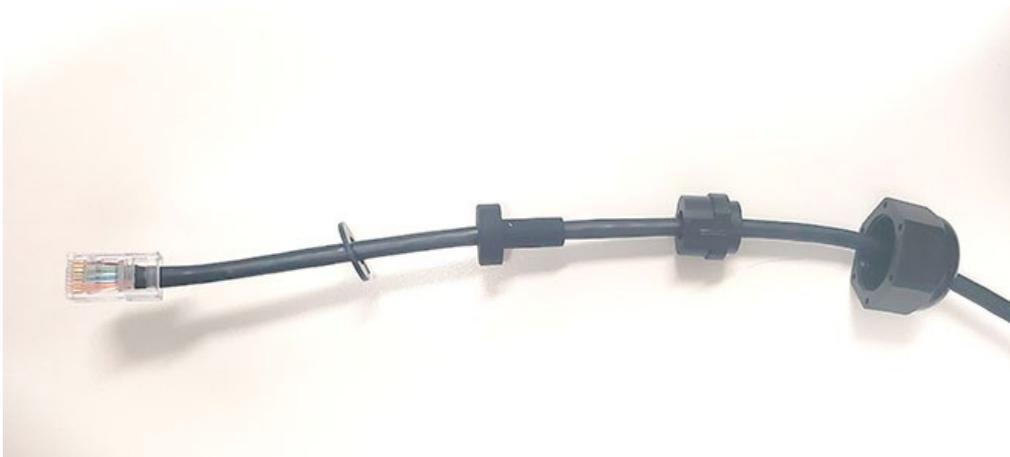
4. Compress the split washer, rubber seal, and spacer so that they fit together inside the cap.
